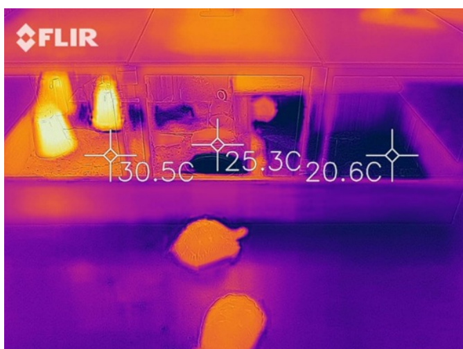
Plate 4-5. Heat gradients within the enclosure, left is the baseline condition whilst right is the experimental. At the time, the ambient temperature in the room was 27°C for both conditions. (Authors own, 2019).
