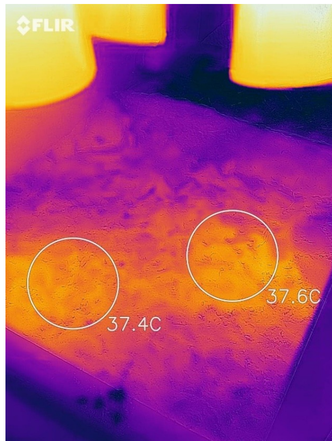
Plate 2-3. Infrared images of the basking spots (zone one) for both conditions. (above) is the baseline (right) is the experimental condition (Authors own, 2019). The CHE bulb was 150W whilst the halogen was 175W; the difference in wattage resulted in a difference in surface temperature; this was minimised by adjusting the height of the bulbs between the conditions.
